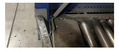
Some Automated Storage and Retrieval Systems (AS/RS) or automated systems specify tighter deflection limits for load beams, such as the length of the beam divided by 240 (or 0.42 percent). This minimizes the risk of the automation (or the load) encountering the beams during loafing or removal.
